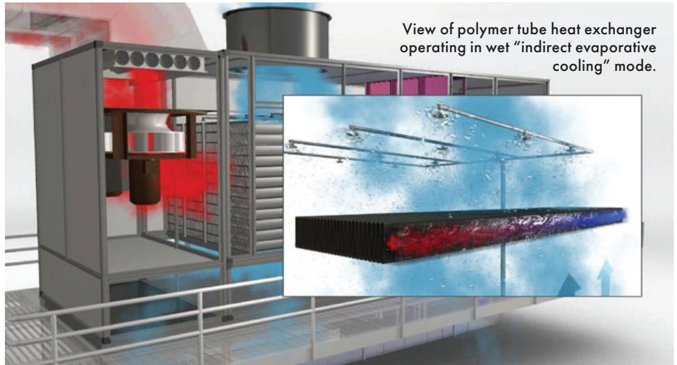
View of polymer tube heat exchanger operating in wet "indirect evaporative cooling" mode.
