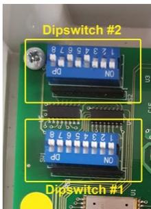
**Dip Switch SW1** is used to set the System ID. This System ID must match the System ID being used by the serial transmitter module in the same control system. The System ID can be set in the range from 0 to 255 using binary. The dip switch numbers conform to the following binary numbers: -
