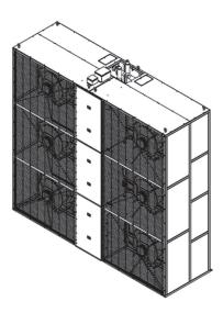
The Modular ChilledWall (MCW 2) data center cooling system comprises modular fan-coil arrays providing incremental cooling capacity options, ranging from 380-550 kW of cooling capacity depending on design temperature change and site altitude. MCW 2 provides options for blow through or draw through fan location, giving designers options that benefit performance or access.
