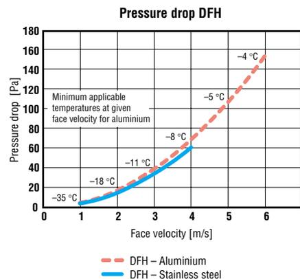
The figure shows the maximum applicable air velocity at a given ambient temperature. The convection of heat strongly increases with increasing air velocity and cools down the surface temperature of the profiles.
