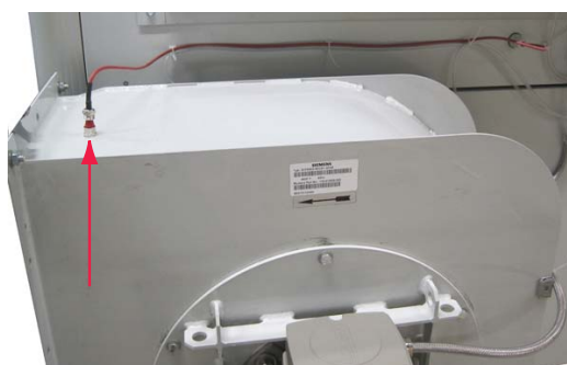
Figure 3.21 PT1000 connection at reactivation fan
