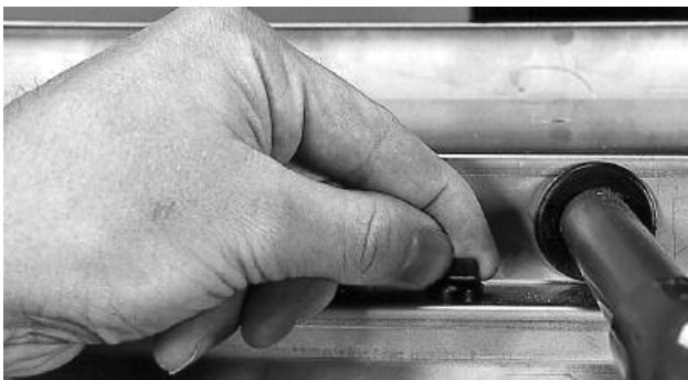
Figure 4.2 Open the safety catch on the distribution header by turning a quarter turn
