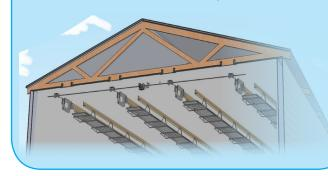
Transition End kit can accomidate 1:1 cable or double back cabling set -up. Includes hand crank.
