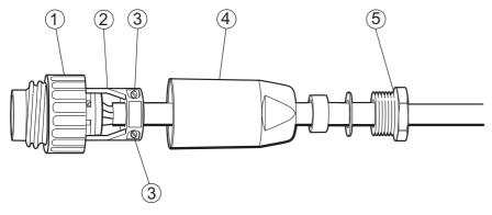
Figure 3.6 Humidistat connection kit assembly
