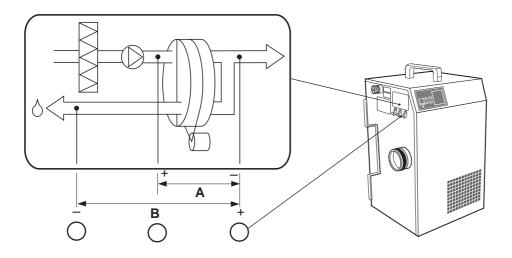
Figure 3.7 Dry and wet airflows/Test points position
