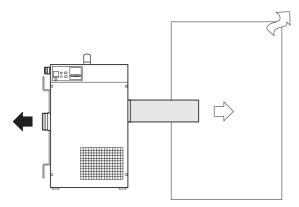
The wet air restrictor plate must be fitted over the wet air outlet when a dry air duct is connected to the unit (length <15 m) and the wet air outlet is freeblowing.
