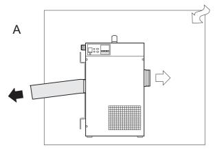
Figure 3.2 Installation in a closed airflow system.
