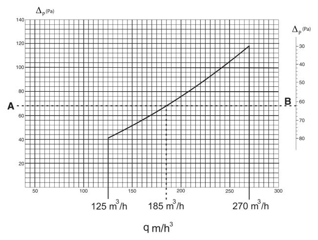
Figure 3.8 Example of required differential pressure curves.
