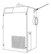
Figure 5.1 High temperature cut-out
