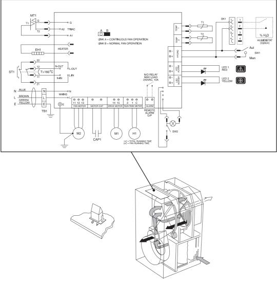
Figure 3.10 Circuit diagram and PCB location
