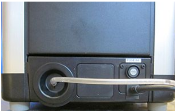
Figure 4.3 Drain hose connection
