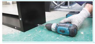
Assemble bottom panel (the one with holes) together with the side panel by means of qty. 1 self tapping screw (round head - 6.3x13), qty. 2 angle brackets and qty. 8 self tapping screws (flat head - 6.3x16).
