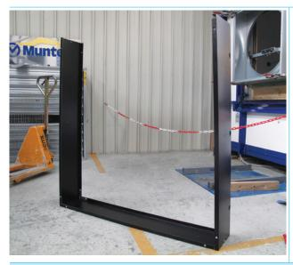
Place the 3 panels set on the floor. The side panel should adhere to the floor.
