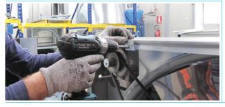
Remove the protection mesh from the back side of the fan and place the hooks on the fan by means of qty. 2 self tapping screws (round head - 6.3x19).
