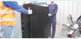
Turn the filter 90° to gain the operating position, with the waves upright.
