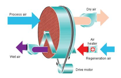
At the heart of the Munters IceDry® solution is our state of the art Desiccant Rotor Technology which has the ability to absorb moisture from the air irrespective of the temperature, so it works equally well even at sub zero temperatures.
