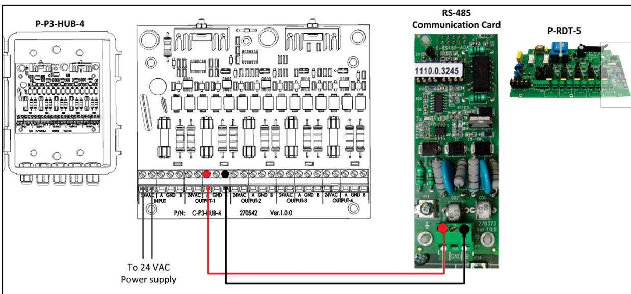
Figure 6: HUB – RDT-5 Thermometer Wiring (RS-485)
