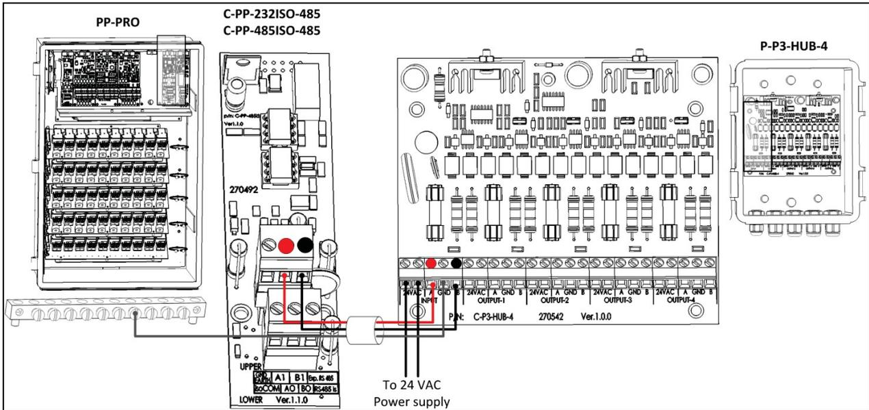
Figure 2: Platinum Pro – HUB Wiring
