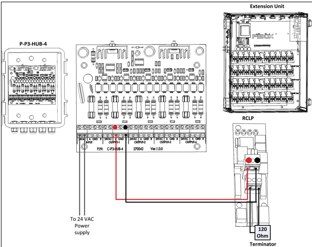
Figure 5: HUB – Platinum Pro Extension Wiring
