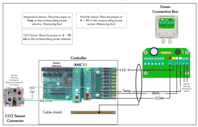
Figure 3: Green Connection Box - Controller RAIC11 wiring (example)
