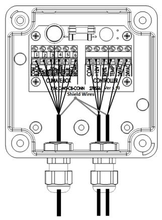
Figure 6: Connection Box shield cables wrap
