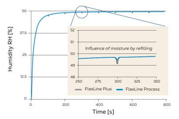
\*Measuring point directly after 2.5 x humidification distance.
