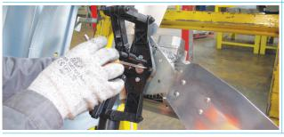
Tighten the screw by using the mm 6 allen key (ref. 17/ Assembling tools).
