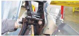
Fix the centrifugal system, the propeller and the hub by q.ty 4 M8×30 hex socket cap screws (ref.45).
