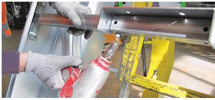
Tighten the nuts by using the screwdriver (ref.3/ Assembling tools).
