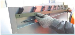
Place the pvc tie-rod (ref. 13) on plastic bearing pivots. Repeat this operation for the other side.
