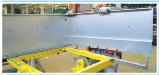
Take the bottom panel (ref.47), the side panels (ref.15-20) and place them taking care that the slot for the plastic bearing is downward.
