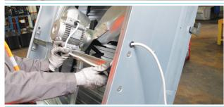
Insert the electric cable into the proper hole placed on the side panel.
