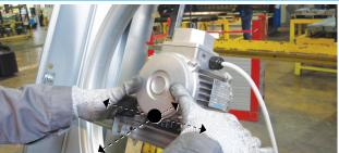
Make sure that the engine is properly centered on the plate and positioned fully forward.
