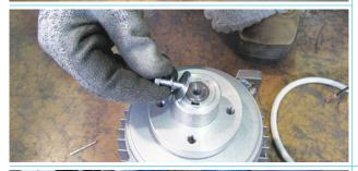
Tighten the screw by using the screwdriver (ref.3/ Assembling tools).
