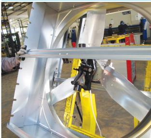
Fix the plastic fork (ref.23) with qty. 2 M6×16 hex screws and qty. 2 M6 thin hex nuts (ref.4-22) on the central shutter blade. Fit central shutter blade on:
