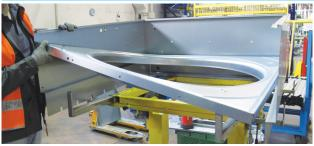
Insert orifice (ref. 19) into the housing on the right side as in the picture.
