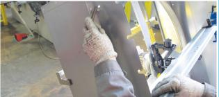
Insert the free terminal of the spring on the hook. Repeat this operation for the other side.
