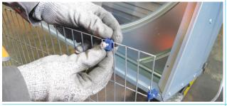
Insert q.ty 12 clips (ref.3) and q.ty 12 Ø6,3×19 screws (ref.3) on the safety mesh guard (ref.31), according to the position of the holes for fixing on the
