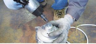
Place the motor on the motor plate and fix it by using:
