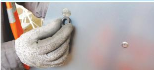
Place the rubber grommet (ref.46) for electric cable protection on the side panel in correspondence with the motor slot.
