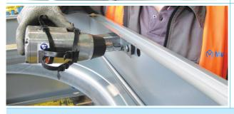
Tighten the nuts by using the screwdriver (ref.3/ Assembling tools) in order to fix the propeller central support to the top and bottom panels.
