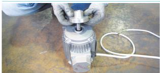
Place the hub (ref. 29) on the shaft of the motor (ref. 32) and fix it by using:
