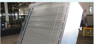
Insert q.ty 6 clips (ref.3) and q.ty 6 Ø6,3×19 screws (ref.2) on the pyramidal safety mesh guard (ref.1), according to the position of the holes for fixing on the housing, and fix by using the screwdriver (ref.3/ Assembling tools).
