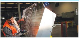
Put the pyramidal safety mesh guard (ref. 1) on the fan as in the picture. The rectangular holes must be positioned horizontally.
