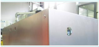
Join bottom panel to side panels and fix qty. 3 pop rivets (ref. 16) for each edge by using the riveting machine (ref. 1/Assembling Tools).
