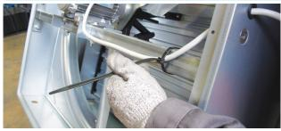
Fix the electric cable to the central support with the clip for motor cable (ref.36).
