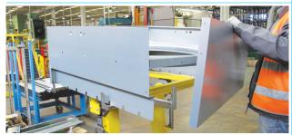
Place the top panel (ref. 18) and fix it to side panels with qty. 3 pop rivets for each side and to orifice with:
