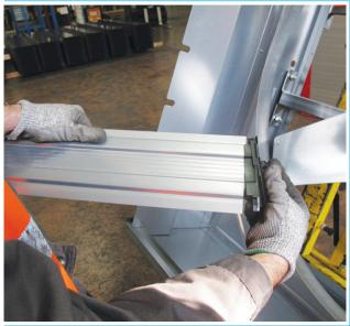
Insert plastic bearings (ref. 7-11) on thin shutter blades (ref. 10) and plastic bearings with spring (ref. 8-12) on central shutter blade (ref. 9 - for ED36HE only).
