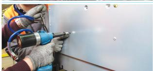
(#) Place M8×17.5 threaded bushes (ref. 17) in correspondence of proper holes around the housing. Qty. 2 long threaded bushes for each panel. Make sure that orifice and each panel are properly joined by the bushes. Use the inserting machine (ref.2/ Assembling Tools).
