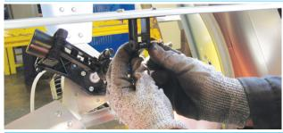
Insert knurled axle (ref.21) by the smooth side on the plastic fork, then take plastic shutter rod on the centrifugal system and fix them together by using a small hammer (ref. 11/Assembling tools).
