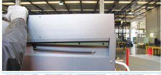
Put cover plate (ref.5) over the plastic bearing mechanism.
