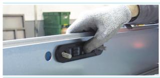
Place the oval plates between propeller central support and panels.
