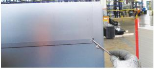
By means of a screwdriver (ref. 14/Assembling tools) insert cover plate over the fan housing.
