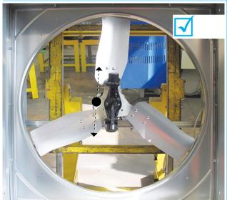
Place the centrifugal system (ref.24) on the propeller (ref.25) and on the shaft of the hub making sure that it is properly oriented.
