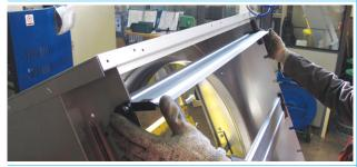
Insert all the shutter blades on the fan housing and then place the fan horizontally.
