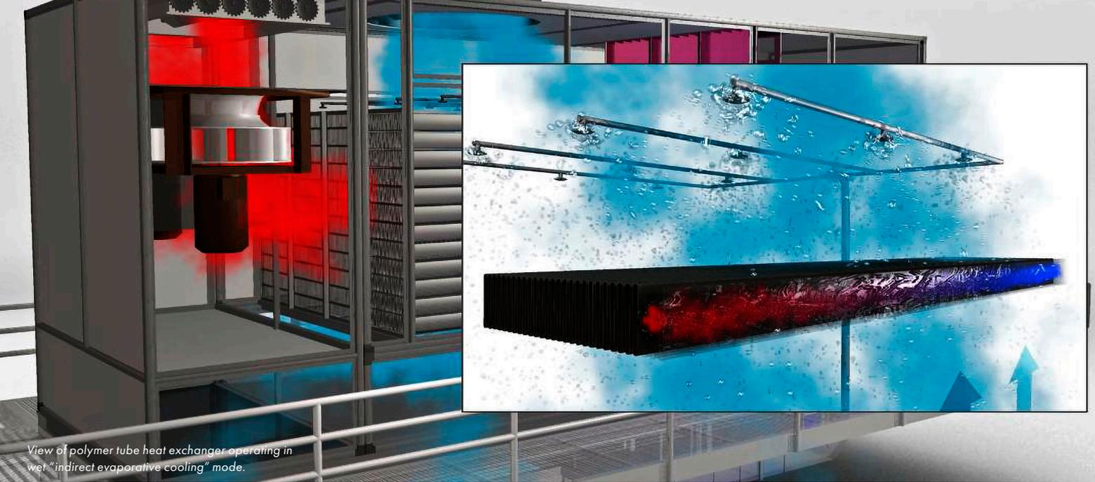
View of polymer tube heat exchanger operating in wet "indirect evaporative cooling" mode.
