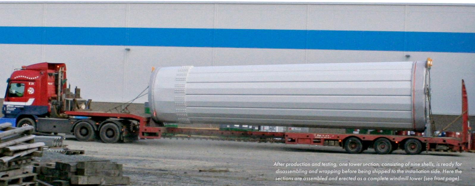
After production and testing, one tower section, consisting of nine shells, is ready for disassembling and wrapping before being shipped to the installation side. Here the sections are assembled and erected as a complete windmill tower (see front page)..
