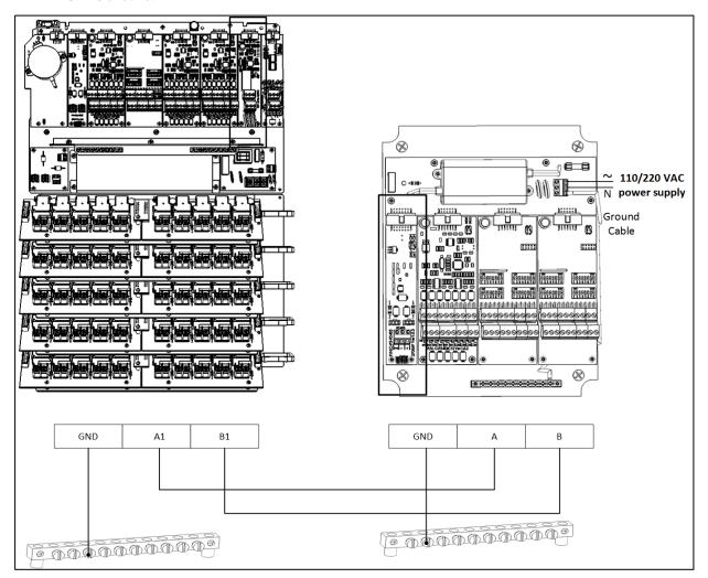
Figure 3: Rotem One to I/O Expansion Wiring / Power cord
