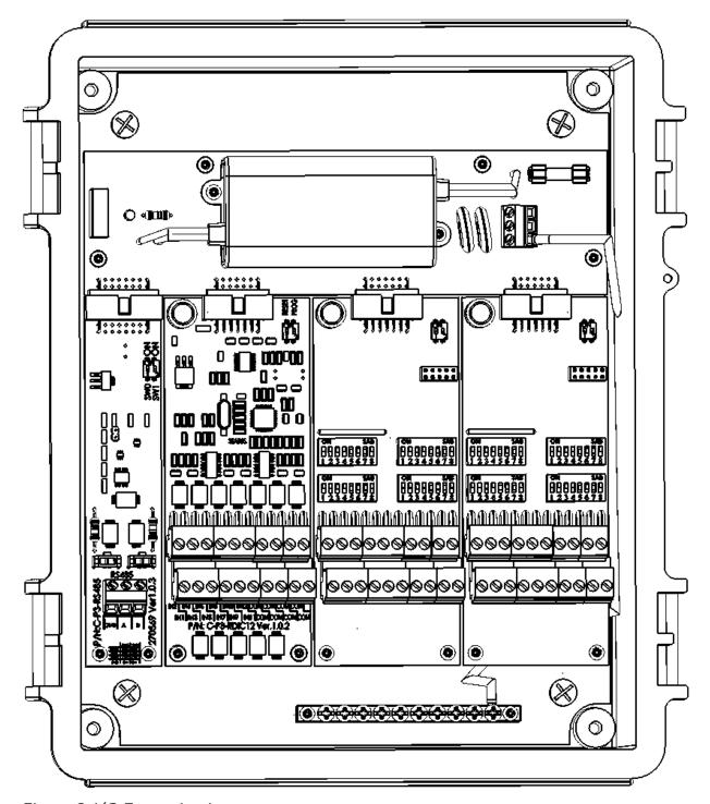
Figure 2: I/O Expansion Layout
