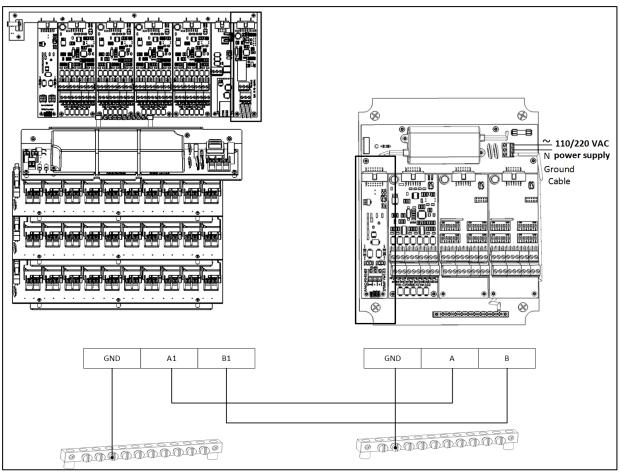
Figure 4: Platinum Pro to I/O Expansion Wiring / Power cord
