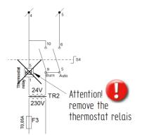
3. Change the settings from the switches on the control unit in the heater. Each heater needs to have its own unique number to be recognised by the interface. The number of the heater can be set by the micro switch S2 on the heater control in the
