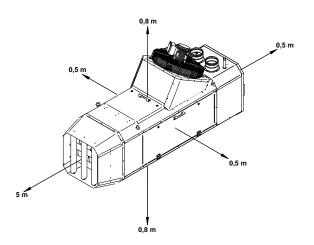
(possibility of) materials within 5m from the front of the heater. See the drawing for the safe distances.
