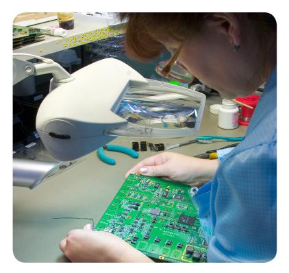
Many sensitive manufacturing processes face problems with static related issues. By providing a climate with constant temperature and humidity, the problem can easily be eliminated. Manufacturing within automotive, electronics and plastic industries, are some examples of areas that benefit from humidification.
