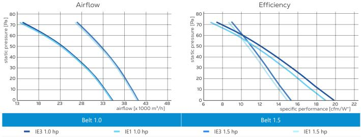
Airflow and efficiency tested in the Munters test chamber in accordance with ANSI/AMCA 210/15 Standard, certified by BESS Lab. \*1 cfm/W = 1.7 ( $m^3/h$ )/W
