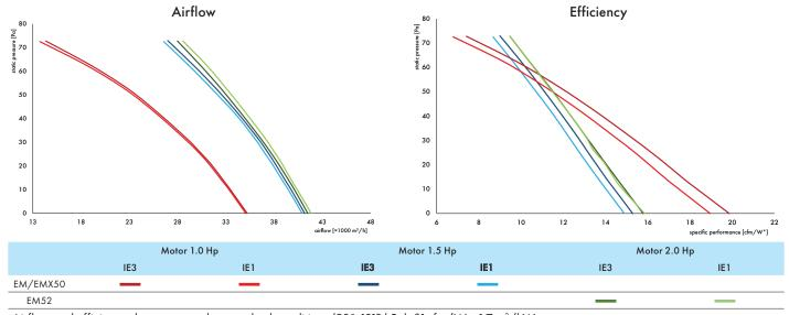
Airflow and efficiency data measured at standard conditions (20°; 1013 hPa). \*1 cfm/W = 1.7  $\,\mathrm{m}^3/\mathrm{hW}$
