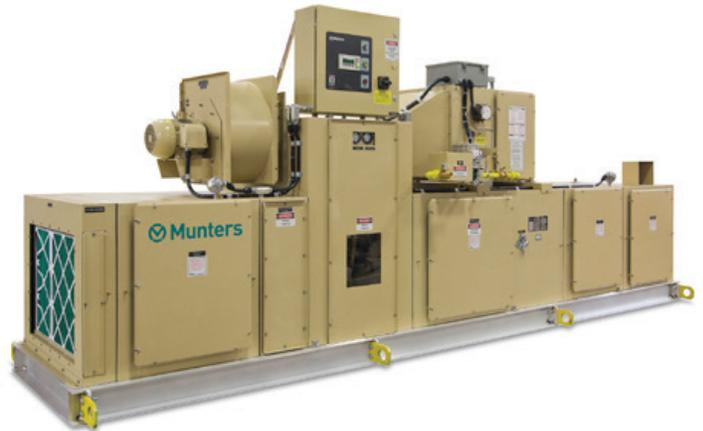
Munters HCD series modular dehumidifiers provide end users the essential dehumidification function in capacities of 600 to 12,000 scfm. Along with the basic HoneyCombe® rotor-drive-and-seal assembly, HCD offers your choice of process and reactivation fan and either gas, steam or electric reactivation.
