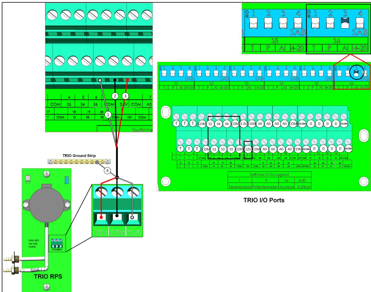
Figure 33: RPS Wiring
