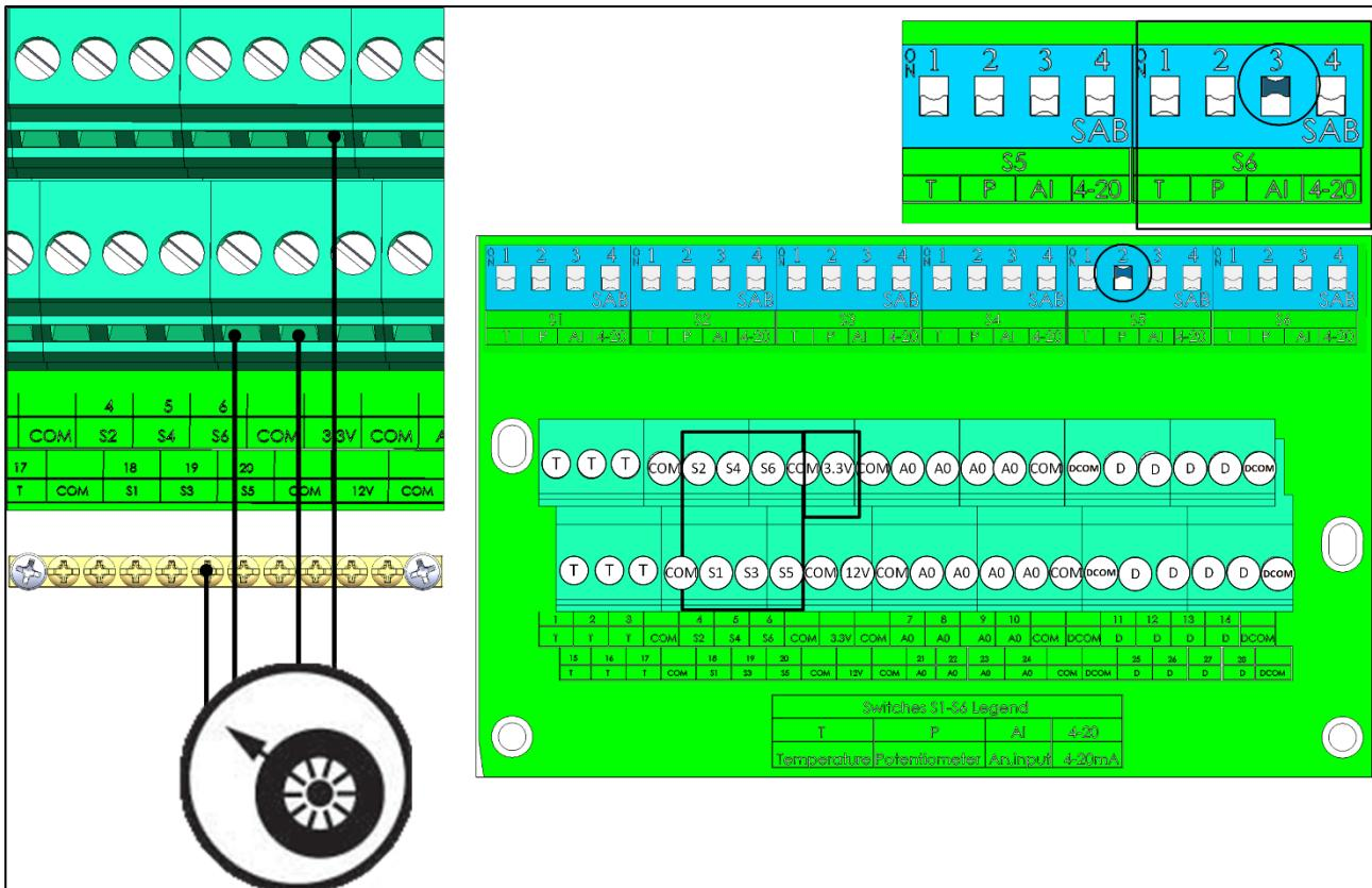
Figure 29: Potentiometer Wiring
