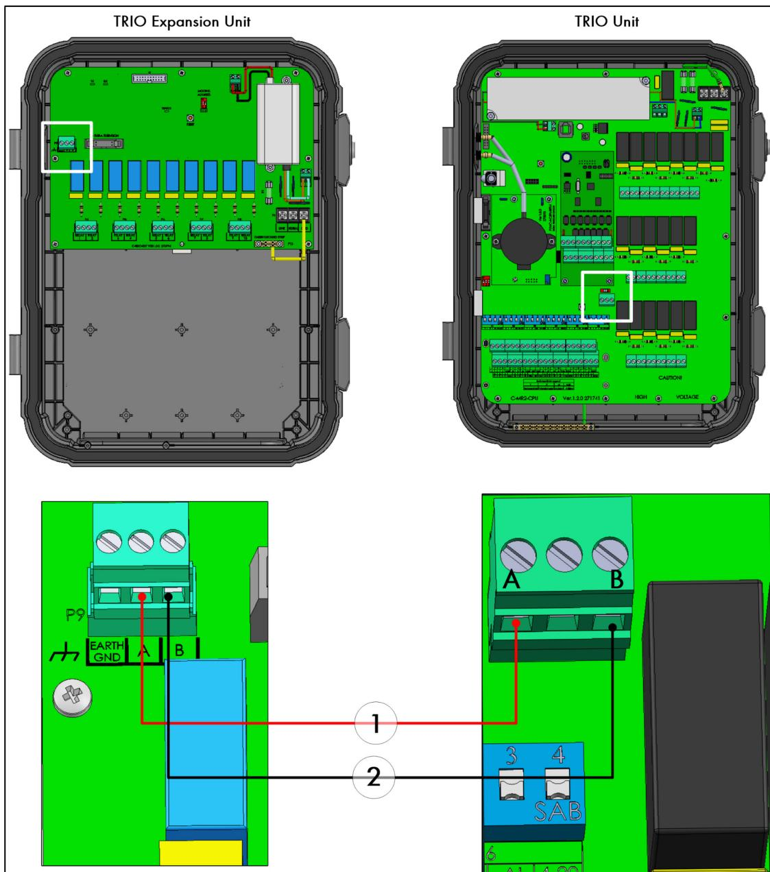
Figure 43: Wiring diagram
