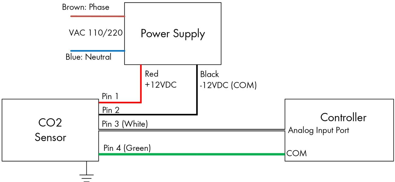
Figure 21: CO<sub>2</sub> Sensor Wiring Schematic
