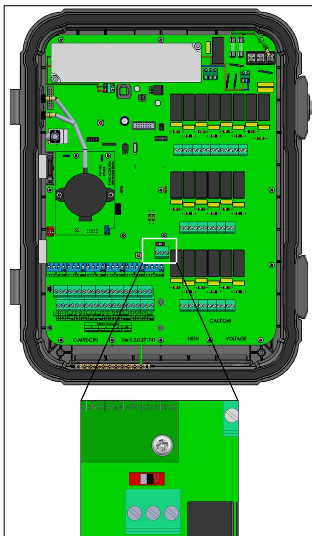
Figure 40: Termination Switch
