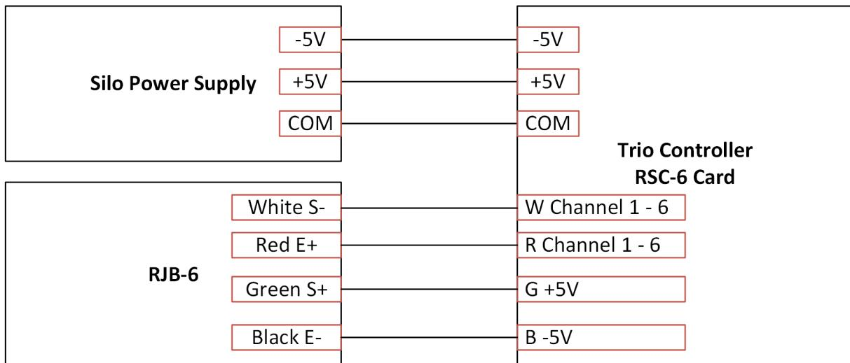
Figure 37: RSC Card to Silo Power Supply/RJB-6 Schematic
