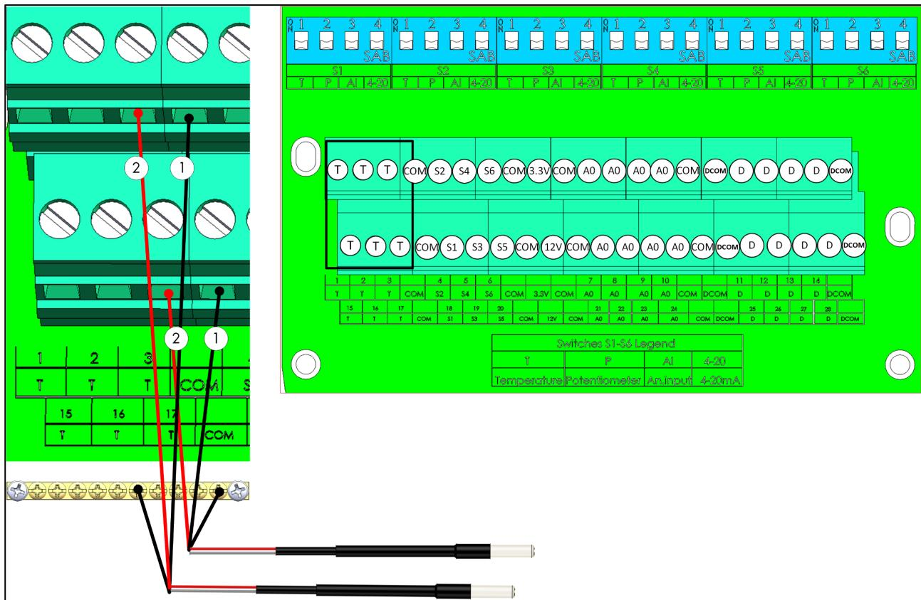
Figure 22: RTS Wiring
