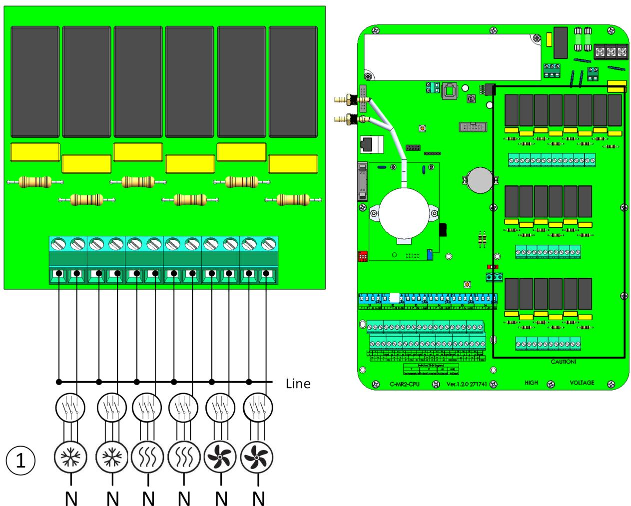
Figure 11: High voltage devices (examples)
