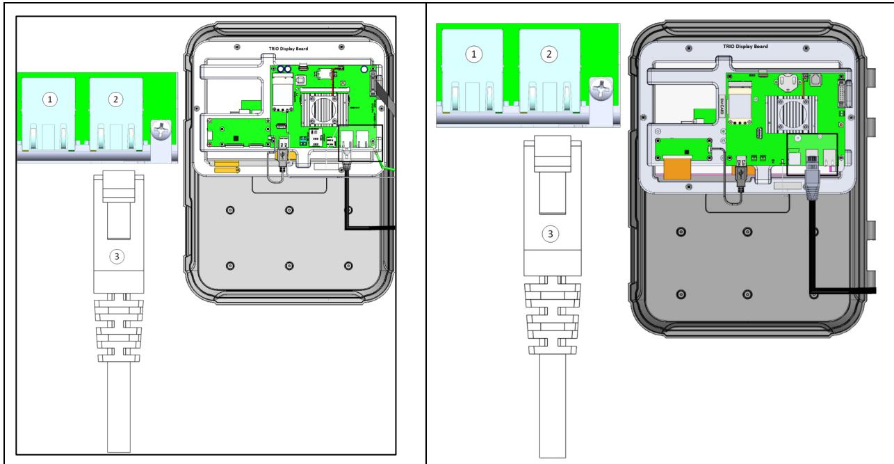
Figure 15: Ethernet port, Display Card Versions 1.0.4 and 1.1.0
