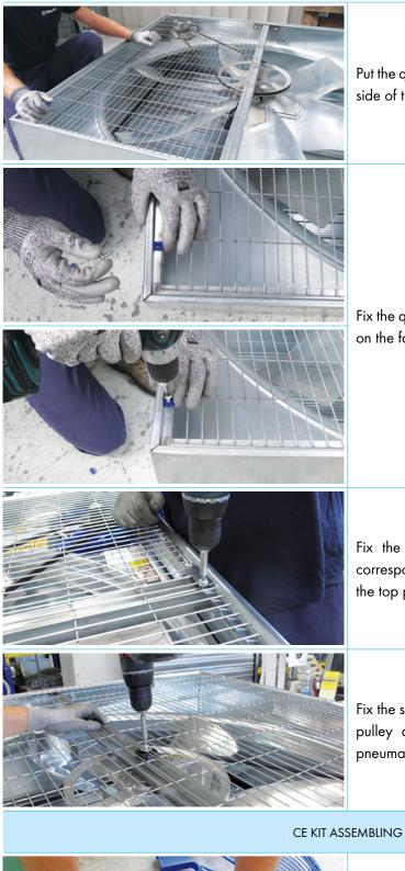
Put the qty. 2 safety meshes guard (ref. 45) on the inlet side of the fan.
