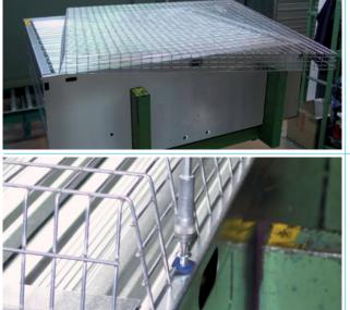
Put the pyramidal shape mesh (ref. 19) on the fan as in the picture. The rectangular holes must be positioned horizontally.
