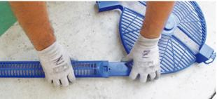
Before assembling the safety meshes complete the CE kit. Join the plastic safety protection for central pulley (ref. 52/A) with plastic safety protection for the V-belt (ref. 52/D).
