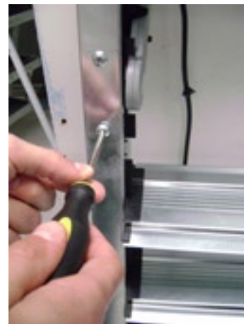
6. Unscrew the two nuts keeping the two halves of the blade together
