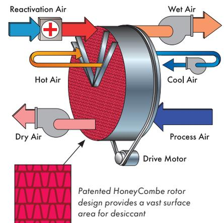
*In the 1950's Munters invented modern industrial dehumidification when it introduced the self-regenerating desiccant rotor, the heart of the dehumidifier.*
