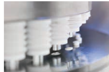
5. Milling & Compressing/Tableting Maintaining the specified humidity set point will result in higher production throughput (prevent product sticking, reduce stoppages, and decrease waste), reduced energy consumption, and improved dosing accuracy.
