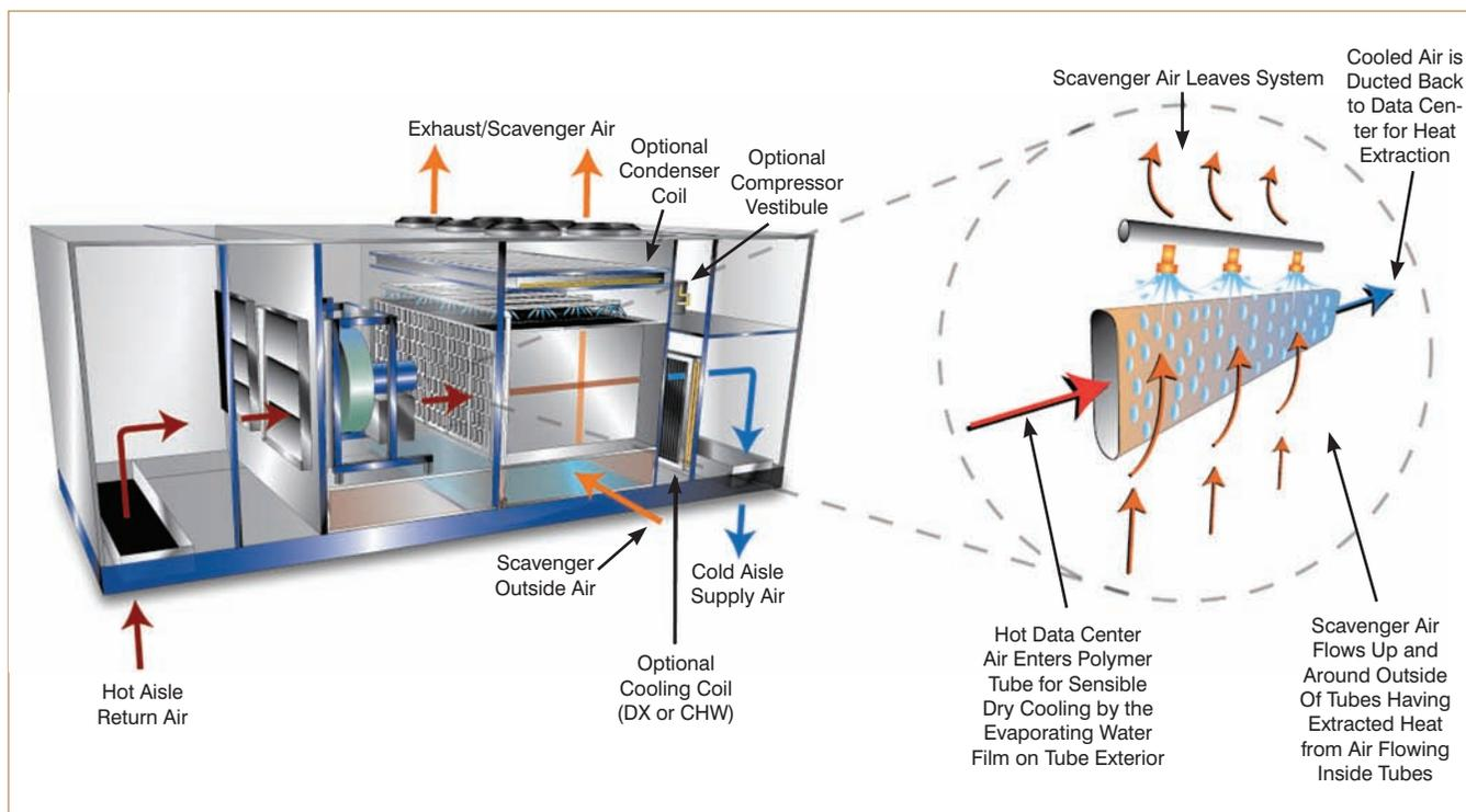
**Figure 3:** Polymer-tube indirect air-side economizer (wet HX).
