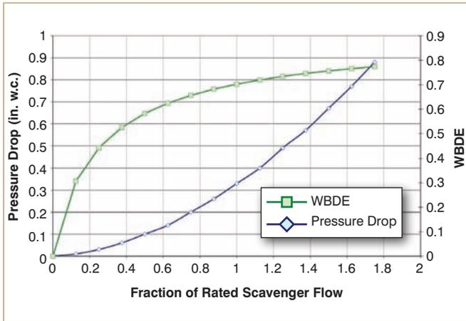
**Figure 4:** Polymer HX performance (wet for IEC) vs. fraction of design rated flow.
