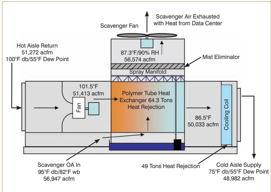
**Figure 7:** Polymer tube IASE system operating in Chicago (673 ft [205 m] elevation) 75°F (23.9°C) cold aisle/100°F (37.8°C) hot aisle. Four units operating to reject a 1,500 kW ICT load. Performance data above applies to one unit.
