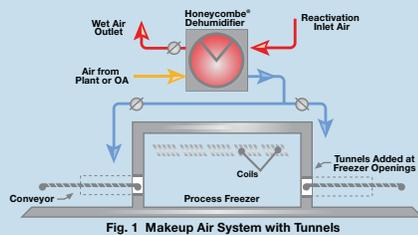
Fig. 1 Make-up Air System with Tunnels
