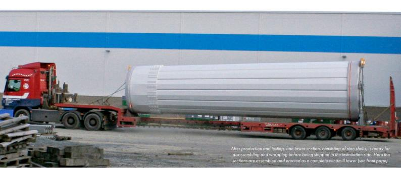
At Andresen Towers in Nyborg, Denmark, Munters desiccant dehumidification protects high quality windmill tower elements before shipping. With Siemens Wind Power, the Danish company Andresen Towers have developed and patented a new type of wind turbine tower built from shells that are bolted together.
