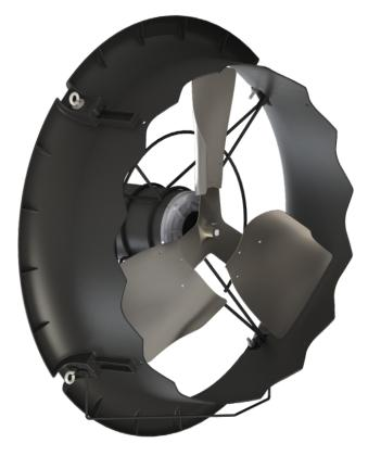
Munters unique chevron design (patent pending) is engineered to minimize specific frequencies generated by the fan blades, reducing noise of the fan in order to provide a comfortable environment for the livestock. Acoustic testing performed in certified, a semi-anechoic chamber to isolate specific frequencies and optimize the design for maximum noise reduction.
