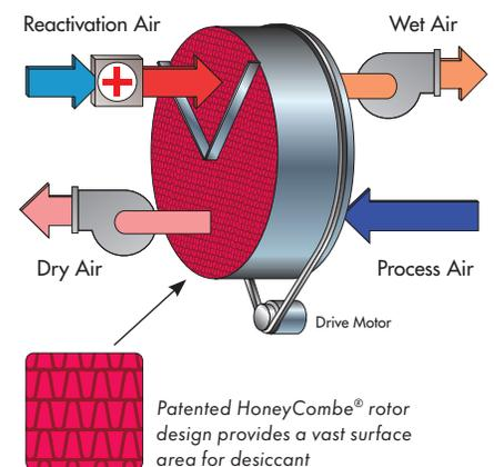
*In the 1950's Munters invented modern industrial dehumidification when it introduced the self-regenerating desiccant rotor, the heart of the dehumidifier.*
