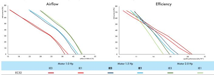
Airflow and efficiency data measured at standard conditions (20°; 1013 hPa). \*1 cfm/W =  $1.7 \text{ m}^3/\text{hW}$
