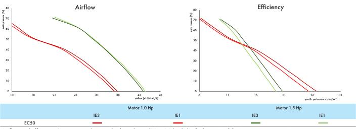
Airflow and efficiency data measured at standard conditions (20°; 1013 hPa). \*1 cfm/W =  $1.7 \text{ m}^3/\text{hW}$
