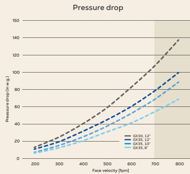
Shaded area indicates the recommended operating range for DropSTOP (above 700 fpm)
