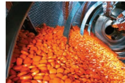
6. Coating Smooth, consistent thickness of coatings yields maximum visual appeal and proper dispersion characteristics. Avoid coating problems like roughness/orange peel, blistering, hazing, sticking and picking, and erosion by selecting and supplying the right drying conditions.
