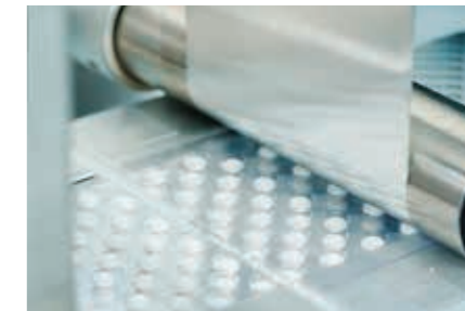
8. Packaging It's not just tablets or capsules that go into blister packing, the surrounding air also gets sealed in. With the right humidity level, you get packaged products that are longer lasting and durable. During blow fill seal packaging, condensation on cold surfaces can lead to surface imperfections that affect appearance and structural integrity. Controlling the dew point of the air around the packaging during the blow forming process can prevent this from happening.
