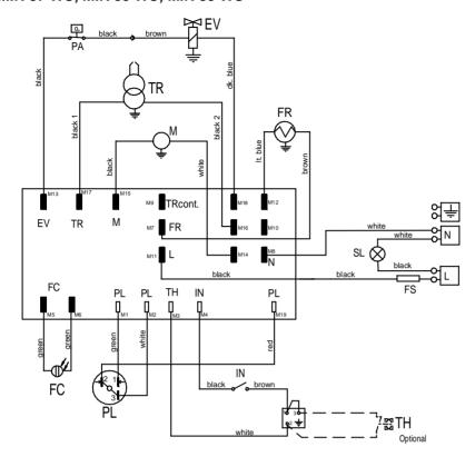
ΕV Fuel Solenoid Valve TR Ignition Transformer
