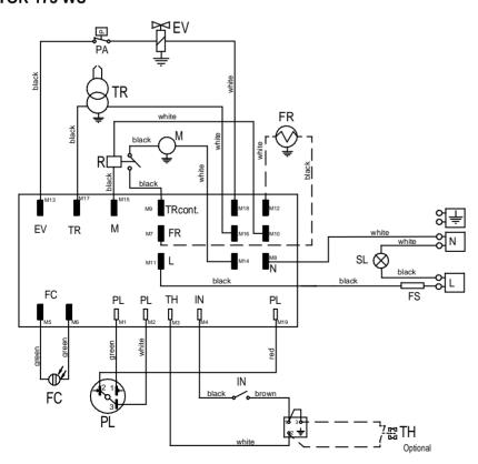
ΕV Fuel Solenoid Valve TR Ignition Transformer
