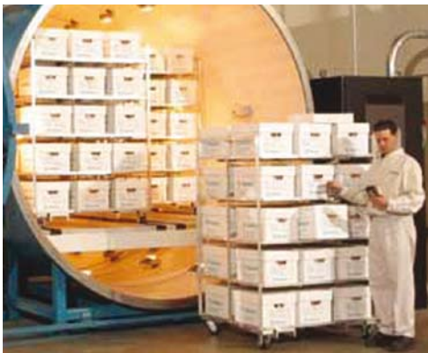
Vacuum drying chamber. The most effective way to dry documents today.
