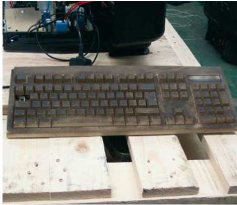
Fire damaged IT system.
