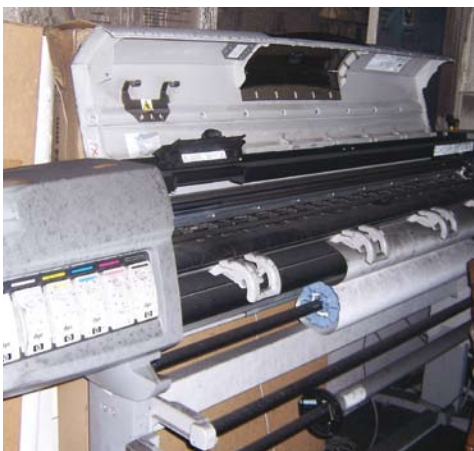
Fire damaged large format printer.
