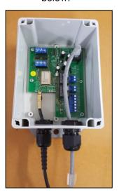
Power to the Transmitter Module is supplied via the Ethernet (LAN) cable. Make sure the power
