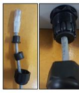
Plug the RJ45 connector on the end of the (one to one) Ethernet (LAN) cable into the socket on
