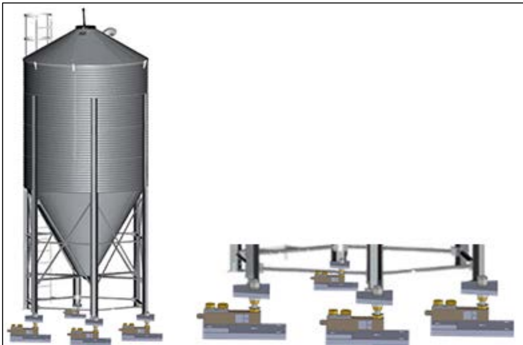
Figure 8: Silo Legs and Load Cells
