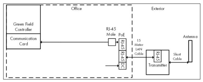
Figure 9: Green Field – G5 Transmitter Block Diagram
