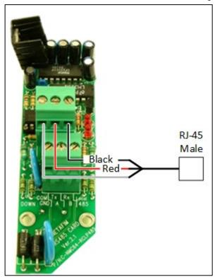
Figure 10: Communication Card Wiring
