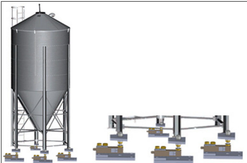
Figure 6: Silo Legs and Load Cells
