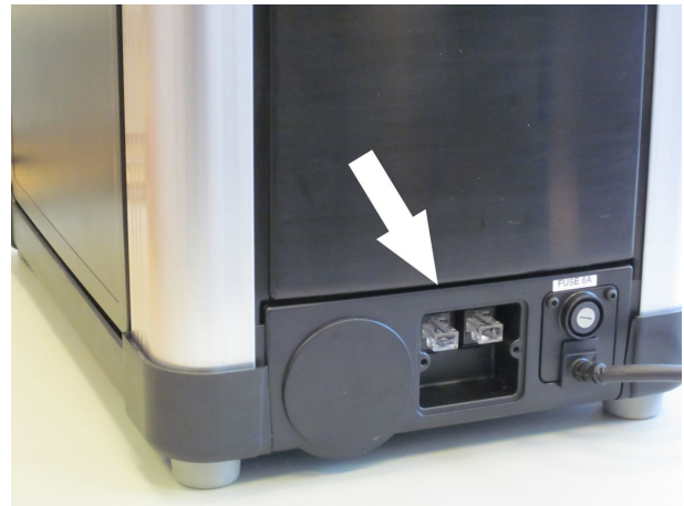
Figure 4.4, 2 CAN BUS ports with empty plugs fitted
