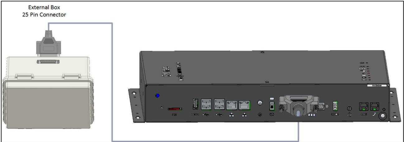
Figura 4: Caja externa - Cable Communicator 2.0
