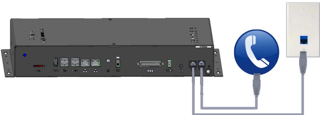
Figure 7: Phone Line Connection
