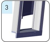
Slide the curved louver in the Bottom header slot
