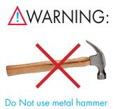
Do Not use metal hammer to secure the MWI. The use of a metal hammer can result in damage to MWI.
