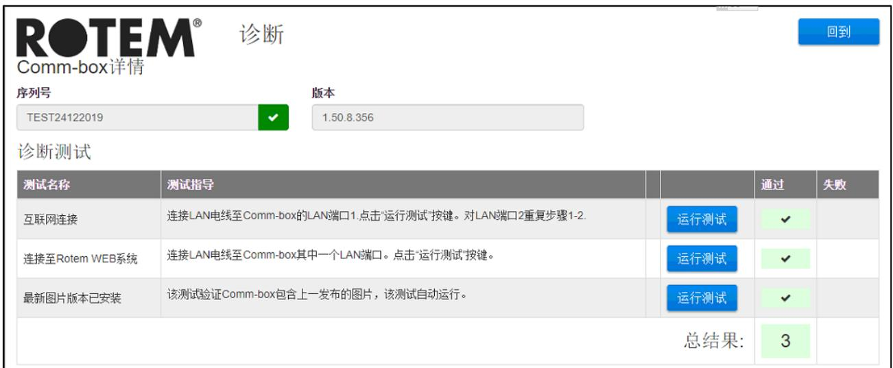
The screenshot shows the 'ROTEM 诊断' (ROTEM Diagnosis) interface. It displays the serial number 'TEST24122019' and version '1.50.8.356'. Below this is a table of diagnostic tests with columns for '测试名称' (Test Name), '测试指导' (Test Instructions), '运行测试' (Run Test), '通过' (Passed), and '失败' (Failed). Three tests are listed, all of which have been passed. A summary row at the bottom shows '总结果: 3' (Total Result: 3).
