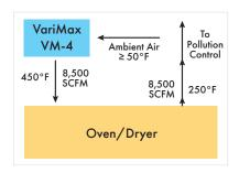
100% O/A oven system provides large temperature rise to a high volume of outside air
