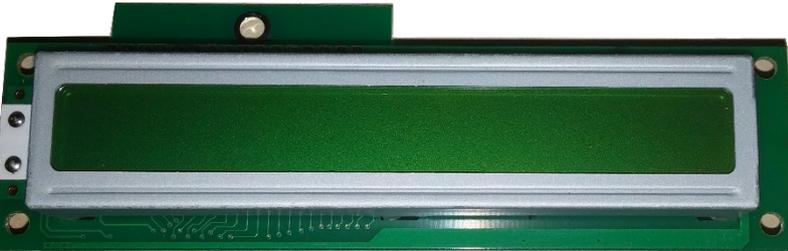
A green printed circuit board (PCB) with a rectangular LCD display in the center. The display is currently blank. The PCB has several gold-colored pins along the bottom edge and a small gold-colored component at the top center.                                                                                          |
