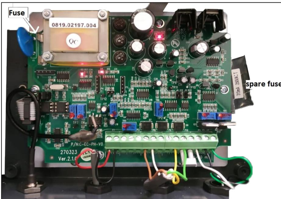
Figura 5: Fuse and spare fuse location
